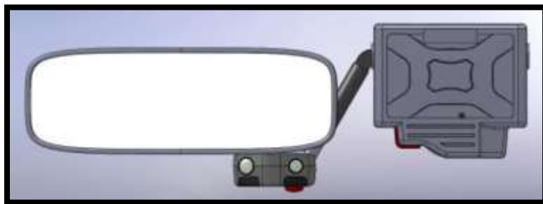
Figure 2. Picture of head unit installed behind rear-view mirror.
