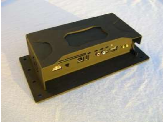
Figure 3. Picture of the main DAS unit which was installed either in sleeper compartment or under passenger-side front seat.
